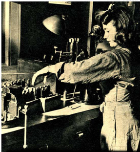
SHE CLEANS AND ADJUSTS A CLIPPER'S 112 SPARK PLUGS.
